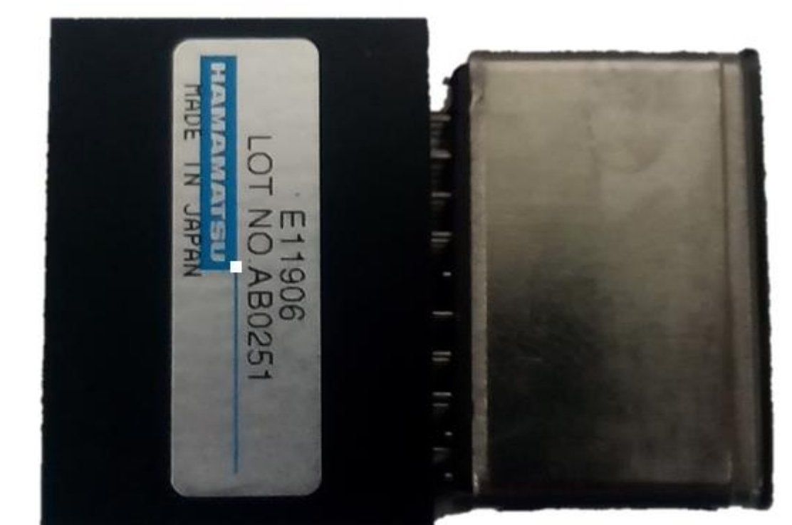
The photomultiplier tube assembled with standard socket from Hamamatsu (E11906)
